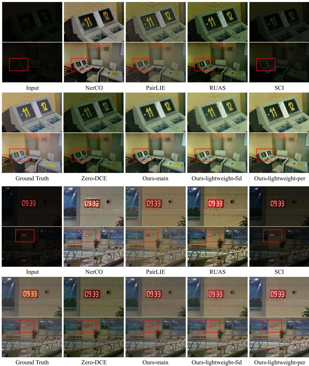
Fig. 11. More low-light enhancement competing results on the LOL datasets with our main and distilled model.
