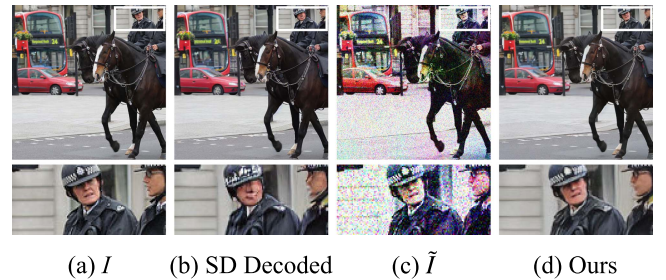
Fig. 5. Structural details preservation with our bypass decoder. (a) Input image I , which results in latent z_0 . (b) z_0 decoded by the SD decoder. (c) The synthesized distortion of I . (d) z_0 decoded by our decoder with encoder features from \tilde{I} as compensation.
